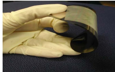
Figure 11a. Prototype FSS structure on flexible substrate.
